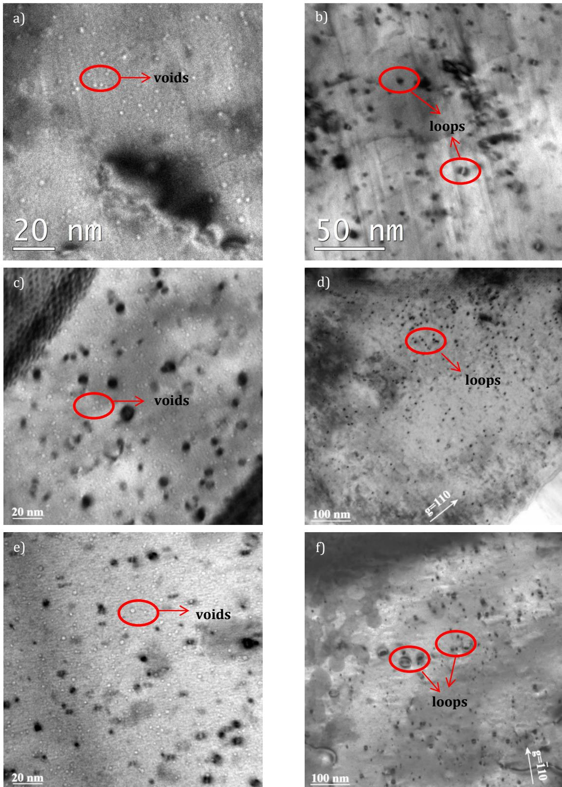
**Figure 1:** Under-focus bright field images showing the presence of voids in the as irradiated at 600 °C (a), PI annealed at 800 °C (c) and 1000 °C (e) forged W bar. Bright field images showing the presence of dislocation loops in the as-irradiated at 600 °C (b) and PI annealed at 800 °C (d) and 1000 °C (f) forged W bar.
