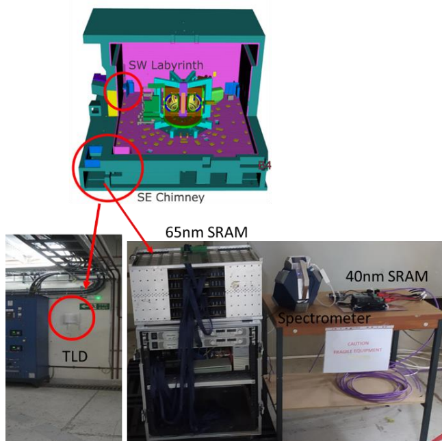
FIG. 16: Picture of the test bench equipped with 65 nm and 40 nm SRAM components and the DIAMON neutron spectrometer as installed in July 2023 in the basement of the south
